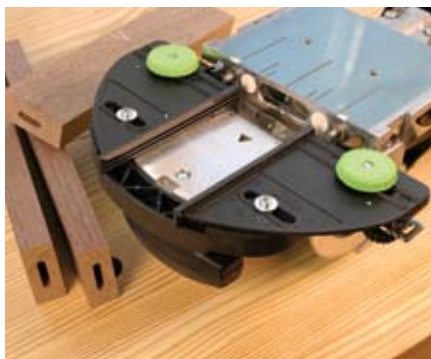
The LA-DF 500 accessory snaps on the fence and allows you make mortises on the ends of thin rails.
