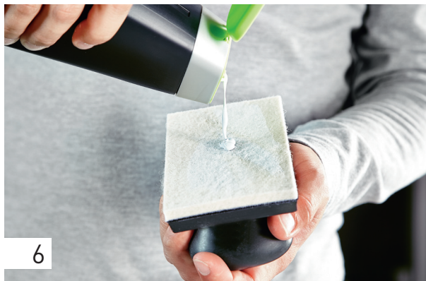
Dab a small amount of MPA 6000 polish onto the polishing felt and rub over the surface.
