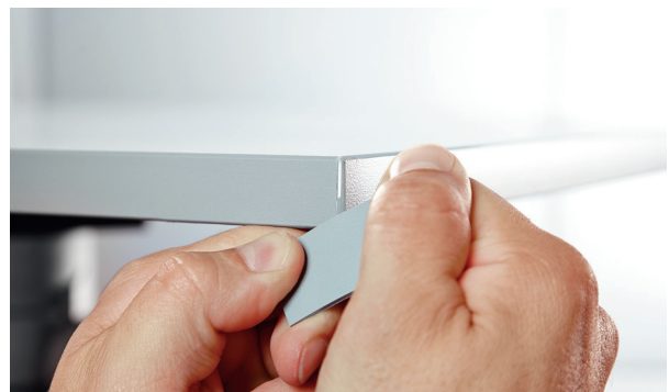
TIP Stress whitening is generated when edging is trimmed. You can remove the whitening simply by rubbing an offcut of edging over the affected area while applying slight pressure.
