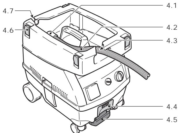
The extractor hose (4.2) is connected to the extractor opening by the angle tube (4.1). During operation, the extractor hose goes through the hose opening (4.3).
